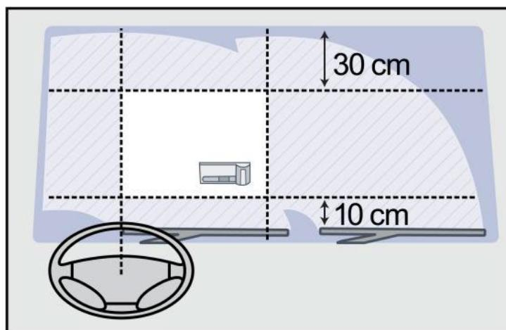
Illustration 21: the correct installation of the GO-Box
